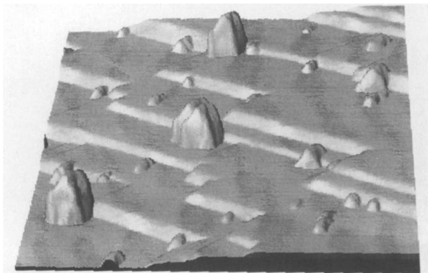
Fig. 3. AFM image ( 8.000 \text{ \AA} \times 8.000 \text{ \AA} ) of sapphire coated with Pt/SB 12 -colloid particles (50 to 60 \text{\AA} high), after annealing in UHV and subsequent calcination in air at 650^\circ\text{C} for 90 min.
