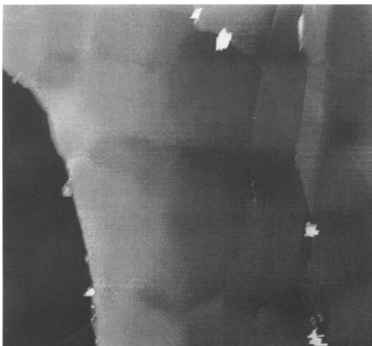
Fig. 2. STM image (10,000 Å × 10,000 Å) of HOPG coated with Pt/SB 12 -colloid particles (70 Å high), after annealing in UHV at 500° C for 30 min.
